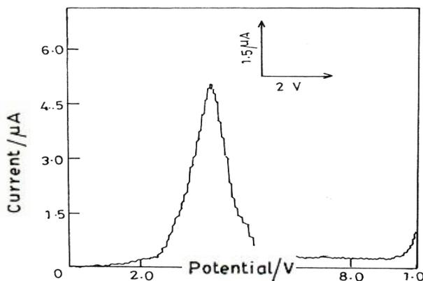
Figure 4: Typical Differential Pulse Polarogram of Cyhalothrin in pH 4.0; Concentration: 0.5 mM, Drop Time: 2 Sec, Pulse Amplitude : 50 mV
