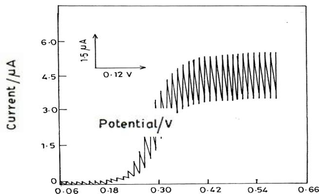
Figure 2: Typical D.C. Polarogram of Cyhalothrin in pH 2.0; Concentration: 0.5 mM, Drop Time: 3 Sec
