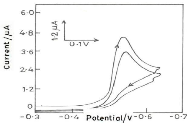
Figure 3: Typical Cyclicvoltammogram of Cyhalothrin in pH 6.0; Concentration : 0.5 mM, Scane Rate: 40  $\text{mVs}^{-1}$
